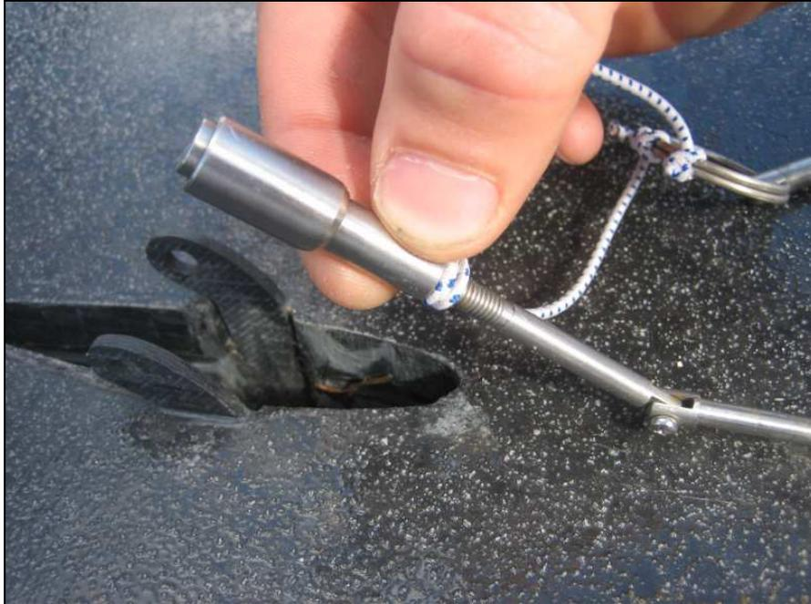
Whilst on the water, you can unclip and wind the ball joint socket head out two full turns until the desired and neutral lift is achieved. Tie your foil retainer pin to the threaded rod adjuster and use this as a guide to see how far you have wound it out.
